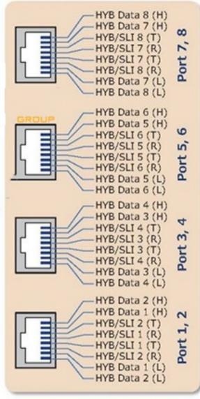
Adapter ADNEC24 – Converts 2 x two port RJ45 sockets to four RJ45 sockets, one port per socket.
