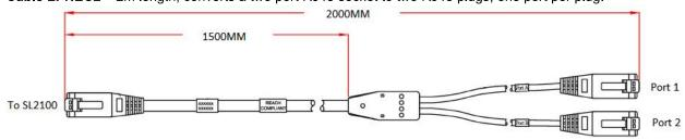
Can be used to connect into an RJ45 through coupler panel or directly into the customer's panels.
