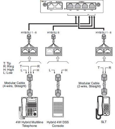
The SL2100 will automatically detected the terminal type when the device is connected.
